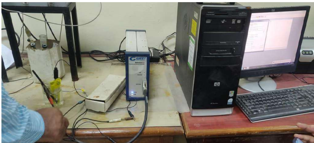
Figure 6: Typical electrochemical corrosion test cell consisting of three electrodes for Potentiodynamic analysis
