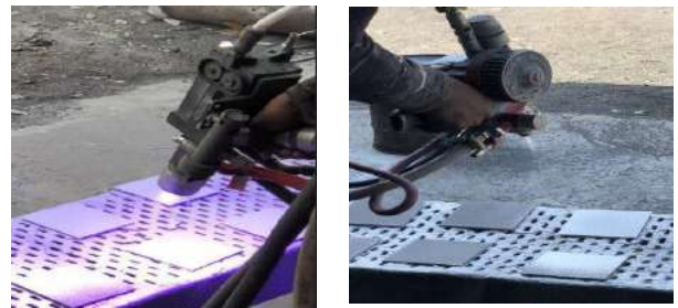
Figure 1: Thermal Spray Coating (Arc & Flame Spray)
