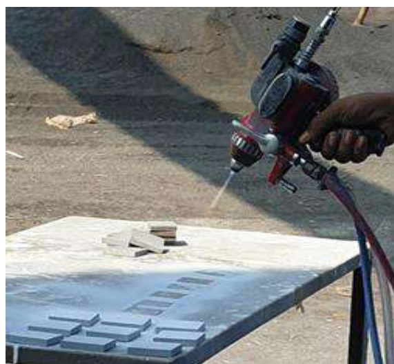
Figure 4: Flame spray system and thermal spray samples
