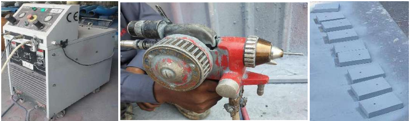
Figure 3: Arc spray system, thermal spray gun and thermal spray samples
