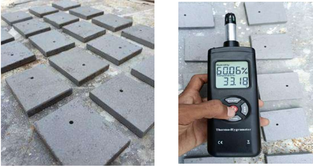
Figure 1: Carbon Steel surface preparation via blasting and humidity testing check
