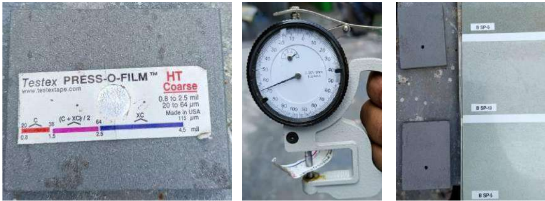
Figure 2: Surface Roughness check by Replica tape and comparing surface profile chart
