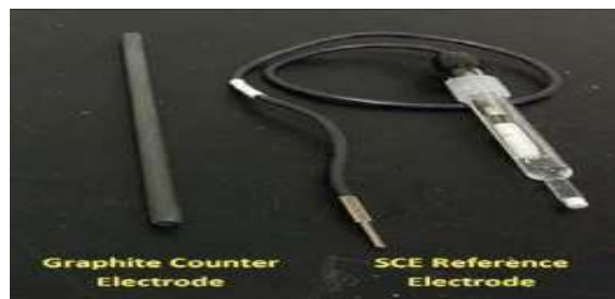
Figure 3: Graphite and SCE electrode
